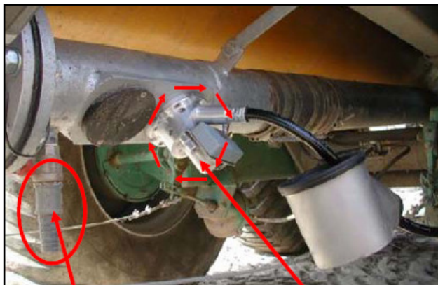
Figure 5: NIR-System installed beneath the liquid manure transport vehicle.
